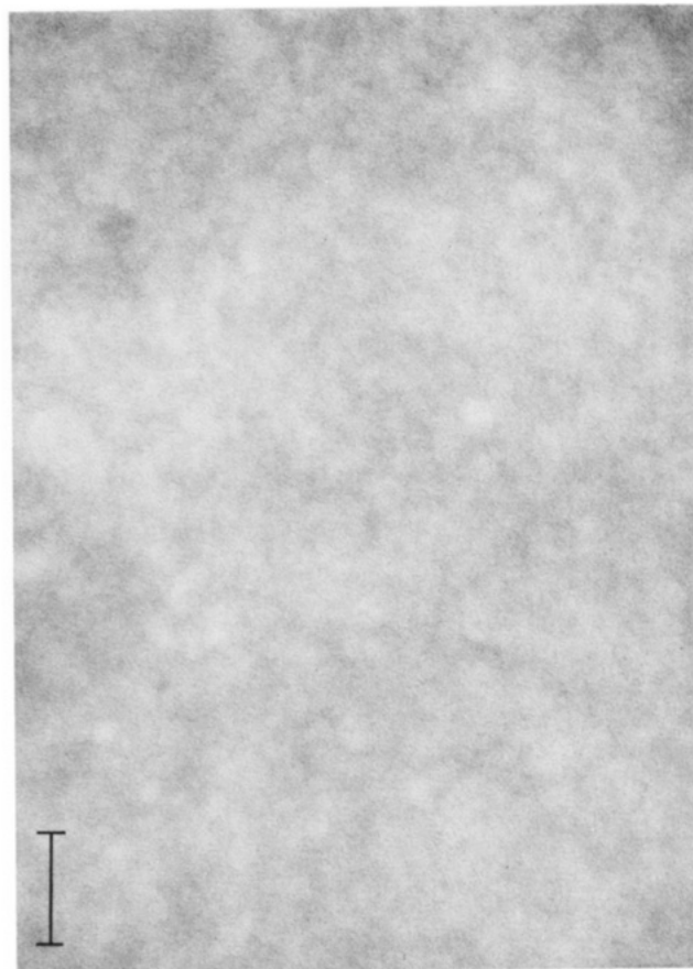
Figure 1. Transmission electron micrograph of an acid catalyzed MEEP/TEOS 50/50 composite. The fiducial line represents a distance of 100 nm.
